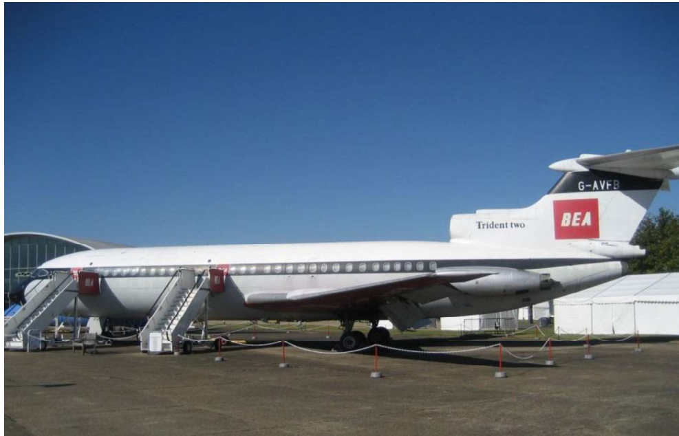
Trident Two at Duxford. Display only. The first series of aircraft to regularly land fully automatically in service. Also the fastest subsonic passenger aircraft.
